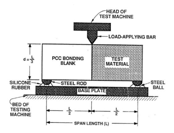
Figure 1 Apparatus for Bonding Strength Test in Center Point Loading
